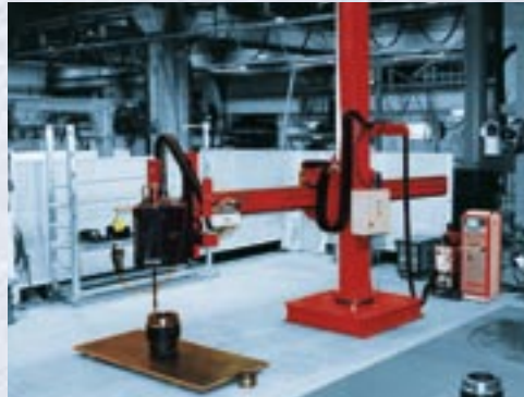
ETR-S overlay welding installation for shipbuilding and onshore/offshore engineering
