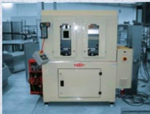
Filter welding installation for automobile industry
