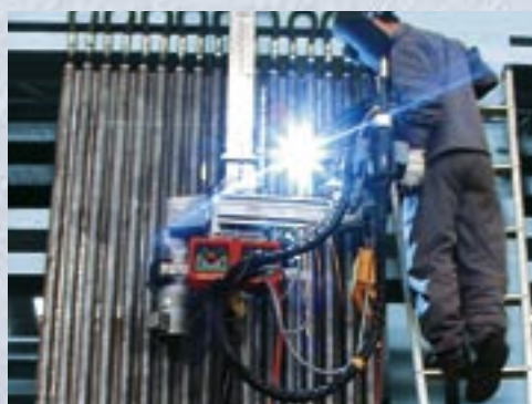
Finned-tube overlay welding installation for use in industrial plant
