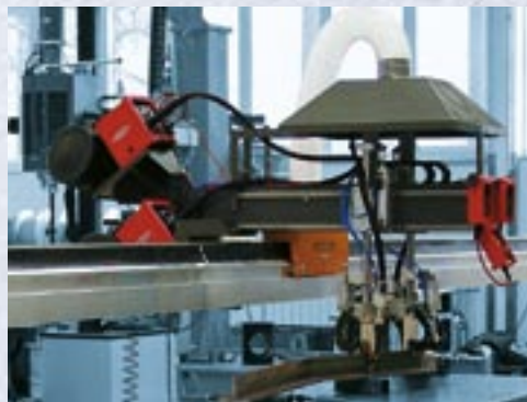
Girder welding installation for custom vehicle construction, bridgebuilding and industrial hangar construction
